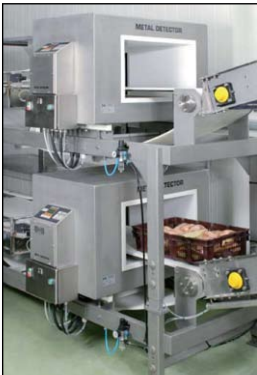
Metal inspection of poultry in E1 containers
